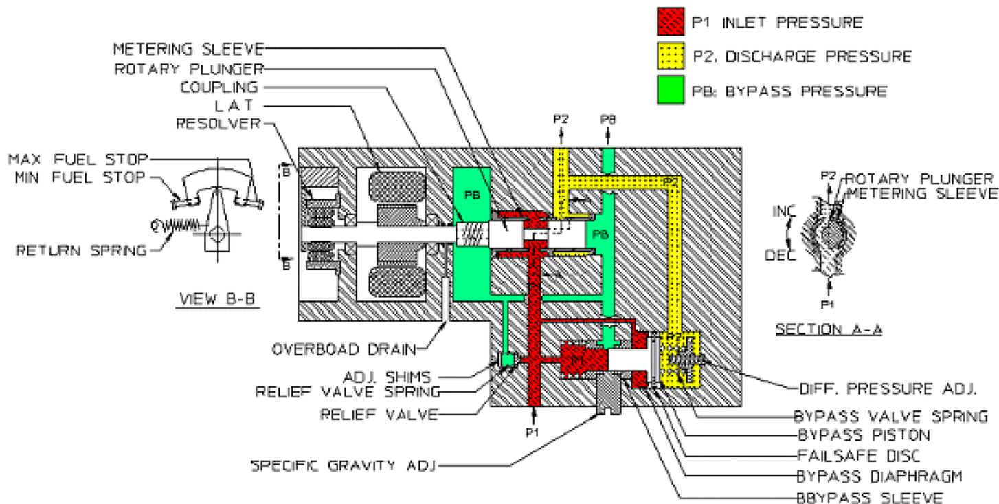
Schematic Diagram – ELV Liquid Fuel Valve
